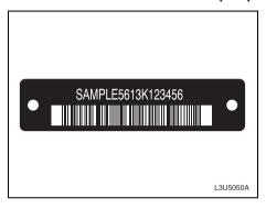
This is the legal identifier for your vehicle. It appears on a plate in the front corner of the instrument panel, on the driver's side. You can see it if you look through the windshield from outside your vehicle. The VIN also appears on the Vehicle Certification and Service Parts labels and the certificates of title and registration.
